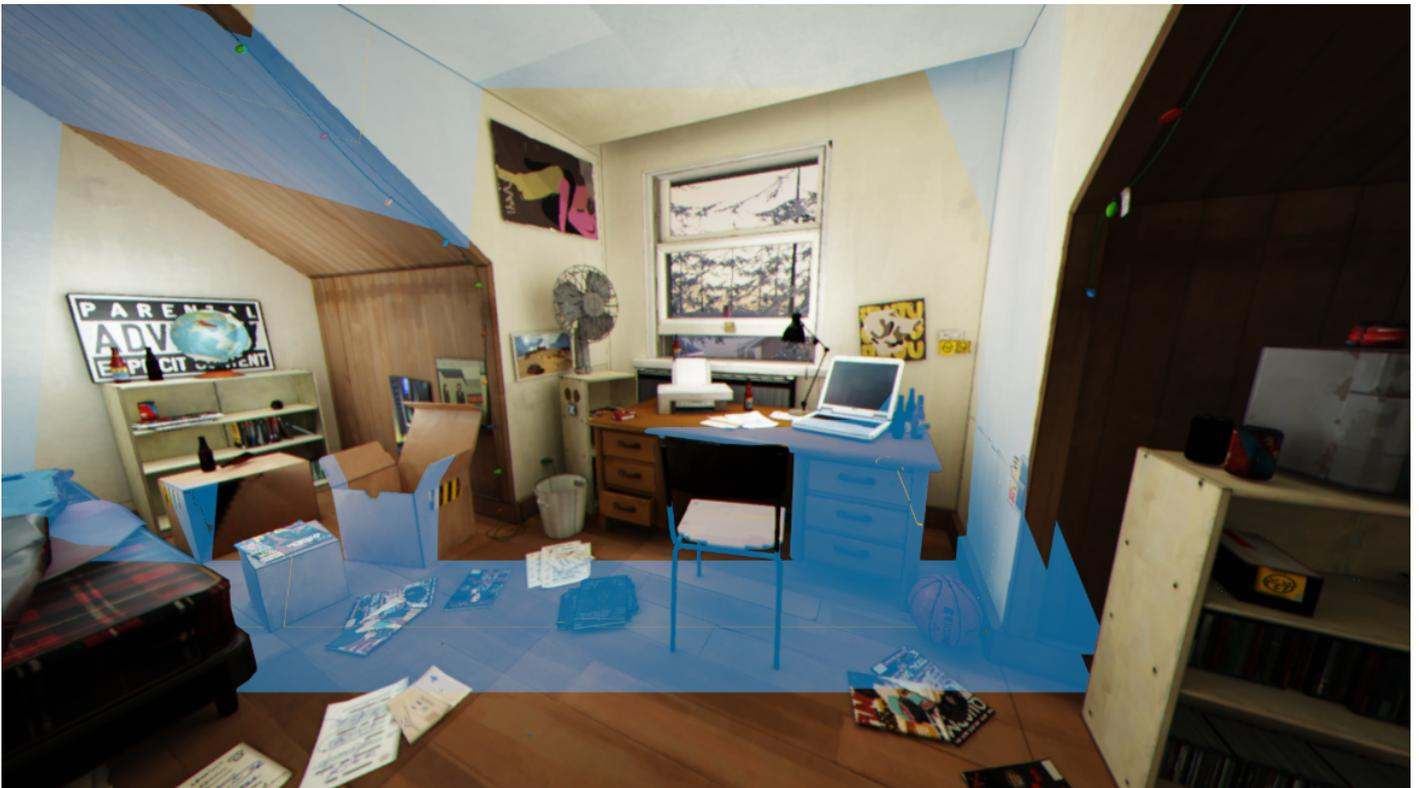
The blue area represents the focal range and the yellow line the focus point. These can be adjusted with the "focalDistance", "focalLength" and "fstop" properties. Make sure to disable this option when you're done.
